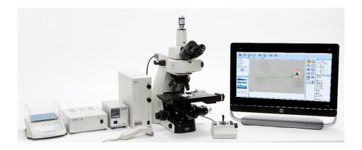
SCA®, CASA System developed by Microptic, is a modular automatic measuring system for the motility, concentration, morphology, DNA fragmentation, vitality and acrosome reaction analysis of semen samples.
